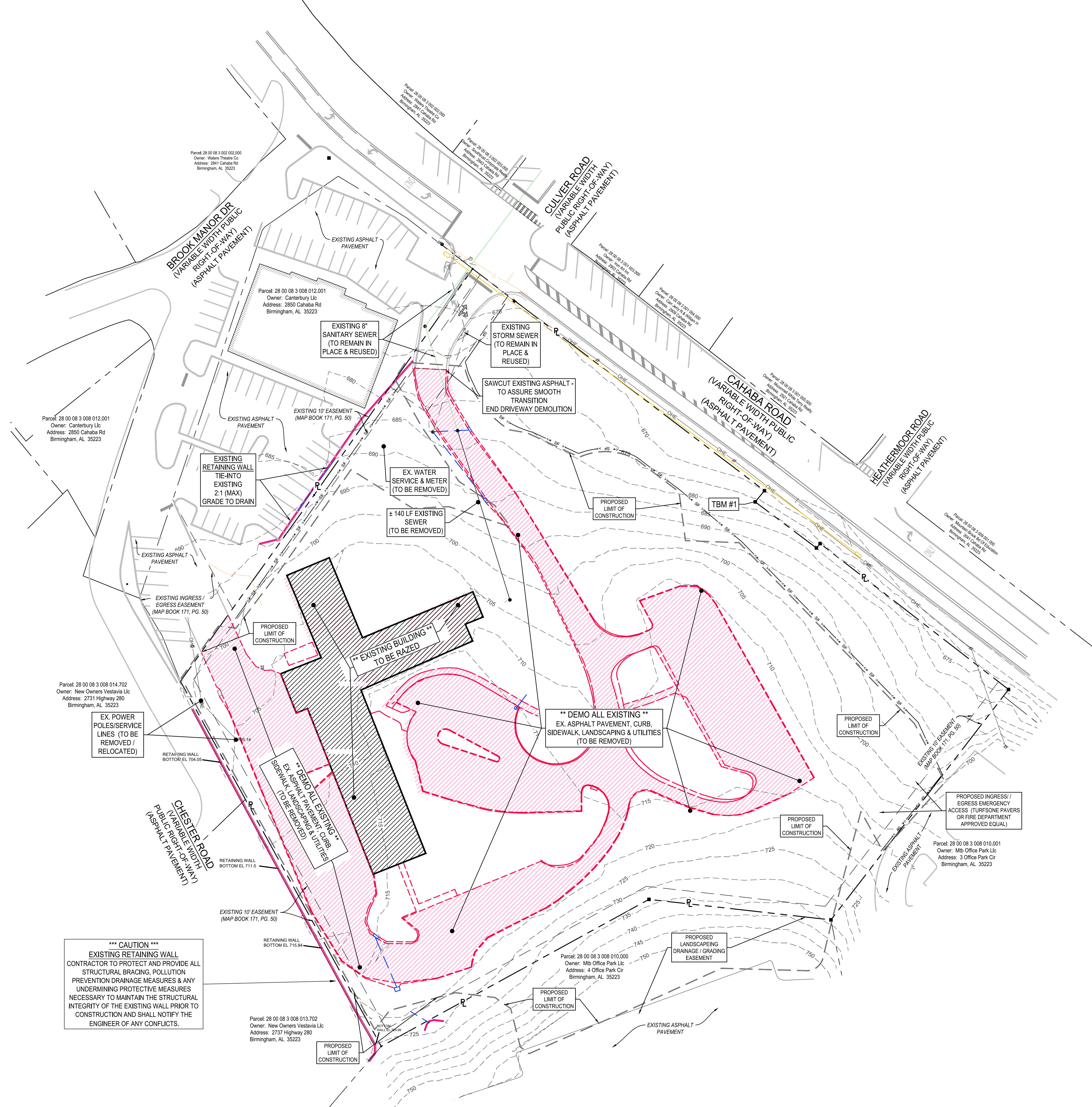
EXISTING CONDITIONS & DEMOLITION PLAN SCALE: 1" = 40'
