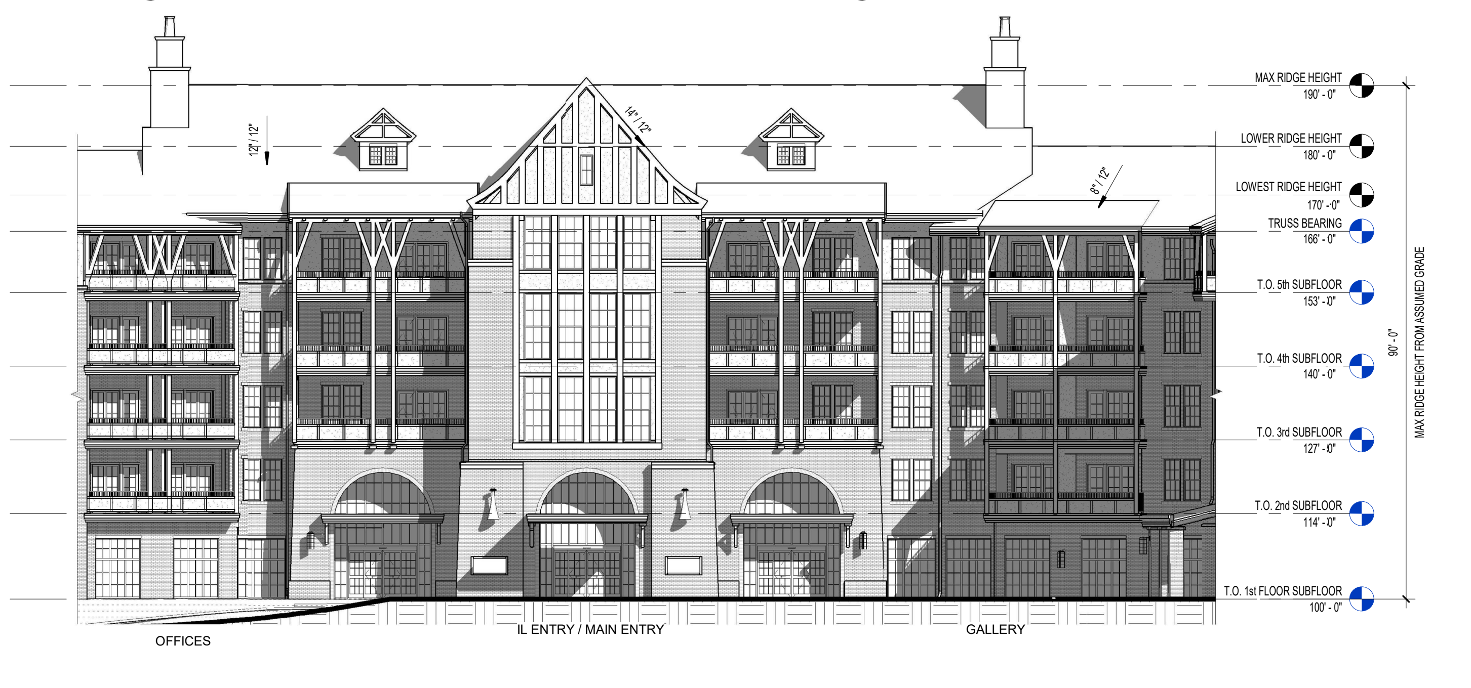
1 NORTH IL ENTRY ELEVATION 1/16" = 1'-0"
